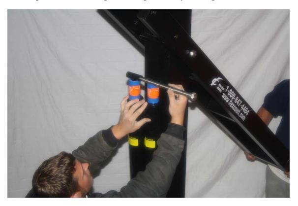
Pull the arm up and use the 18mm x 11" bolt and connect the pistons as shown
