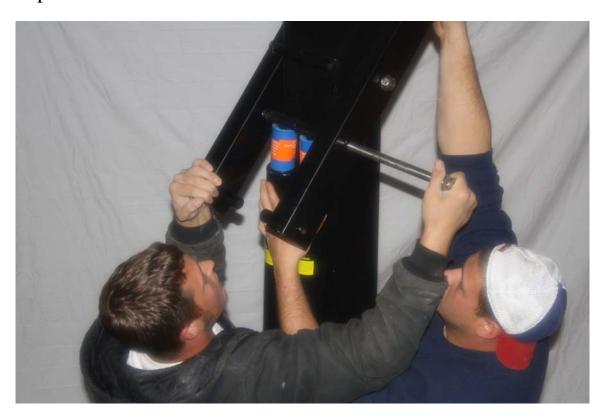
Connect the Bottom of the crank with the 12mm x 4.5" Bolt and Nut  $\,$
