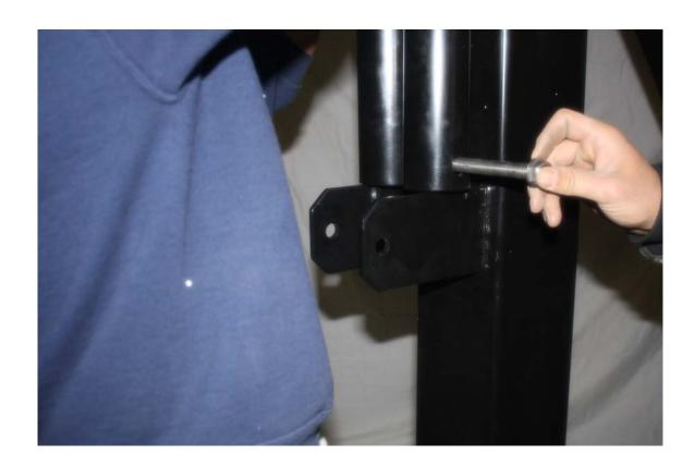
Tip: When connecting the top of the pistons, if the holes don't line up, use a bolt to spin the tops so they line up as shown
