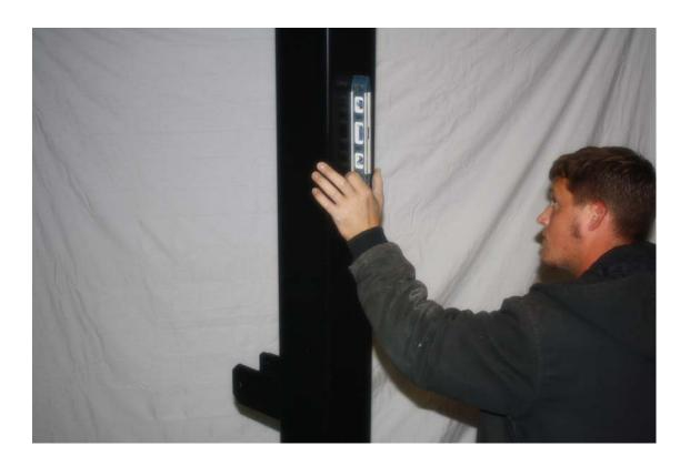
Attach Lower Extension Arm with 16mm x 11" Bolt and Nut. NOTE: Use the First Set of Holes on the extension arm
