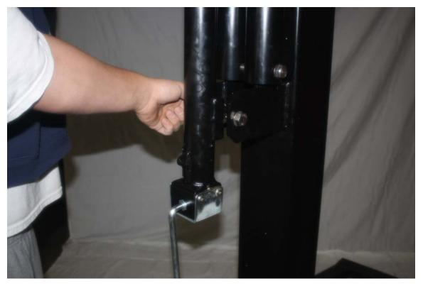
Adjust the Crank up to match the holes and fasten the crank down with the 16mm x 11" bolt and Nut
